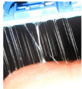
The claim is that viscoelasticity of the fluid alone does not give rise to a small satellite bead between two much larger beads, but that inertia is also required to develop this morphology. The seminal work of Boys [3] demonstrated the formation of BOAS morphology by a viscous Newtonian fluid surrounding a central rigid core driven by capillary action.
